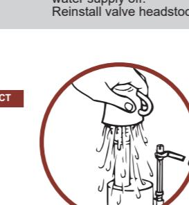
**e3** With the help of a pin, remove the filter. Let the water run until the dirt is removed.
