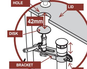
**d** Turn threaded rod to 90 degree and pull up. Release the clip then move and adjust the float height and water level as your requirement.
