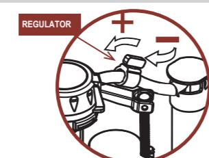
**c** To adjust the water flush, use the lateral gates.
