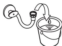
**b** Adjust the water flow with regulator according to the amount of water required by toilet for the hydraulic seal.
