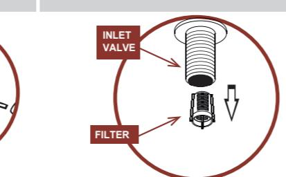
**e3** With the help of a pin, remove the filter. Let the water run until the dirt is removed. Reinstall valve headstock.
