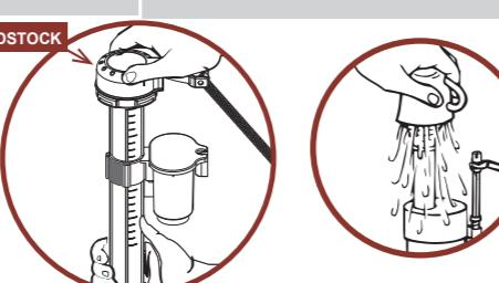
**e2** While holding a container over the uncapped Valve to prevent splashing, turn water supply on and off a few times. Leave water supply off. Reinstall valve headstock.
