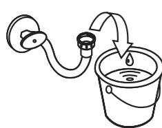
**b** Adjust the water flow with regulator according to the amount of water required by toilet for the hydraulic seal.
