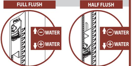
**d** Turn threaded rod to 90 degree and pull up. Release the clip then move and adjust the float height and water level as your requirement.
