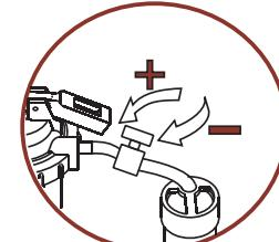
**c** Use the screwdriver to adjust the water level.
